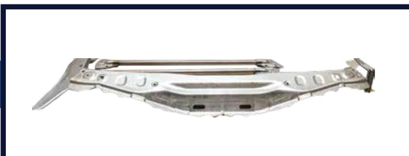
**ASSEMBLY PARTS INCLUDING DOOR IMPACT BEAMS**
